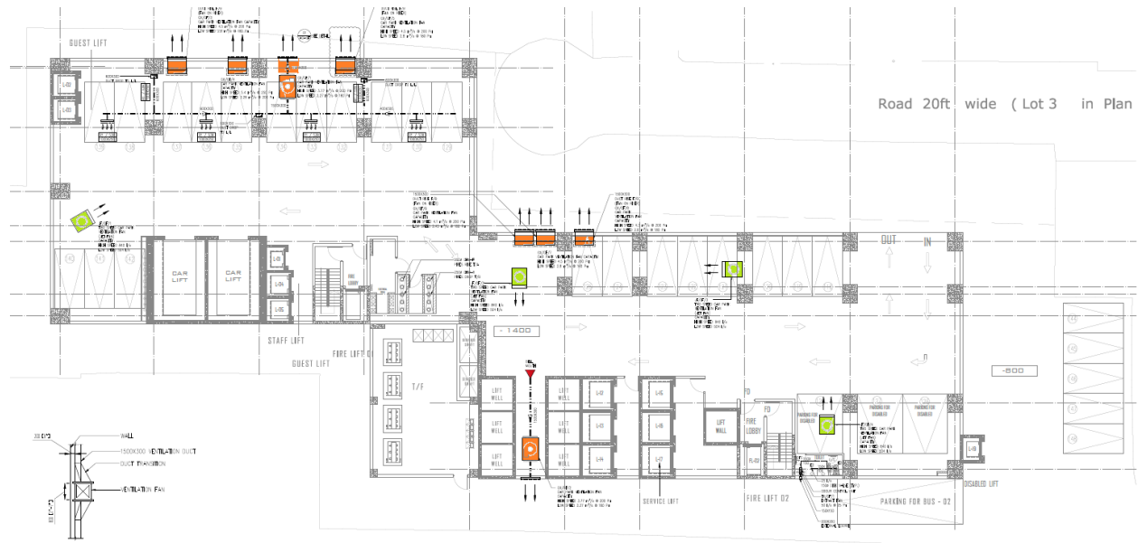
Figure 2.11: Ground Floor Inflow (Inflow) and Exhaust (Orange) Vents
