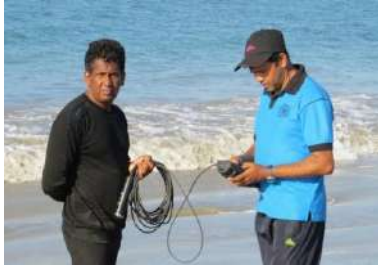
Figure 2-5: Multiparameter reader (YSI Pro Plus) used to measure Physico-chemical parameters
