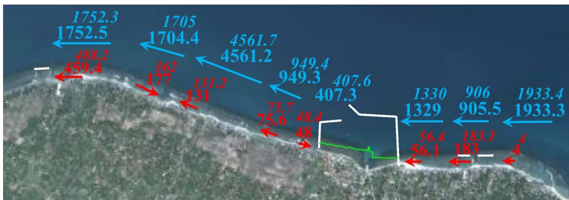
Figure 4-7: Summary of the sediment transport associated with the coastal waters adjacent to Point Pedro Fisheries Harbor (EML, 2018)
