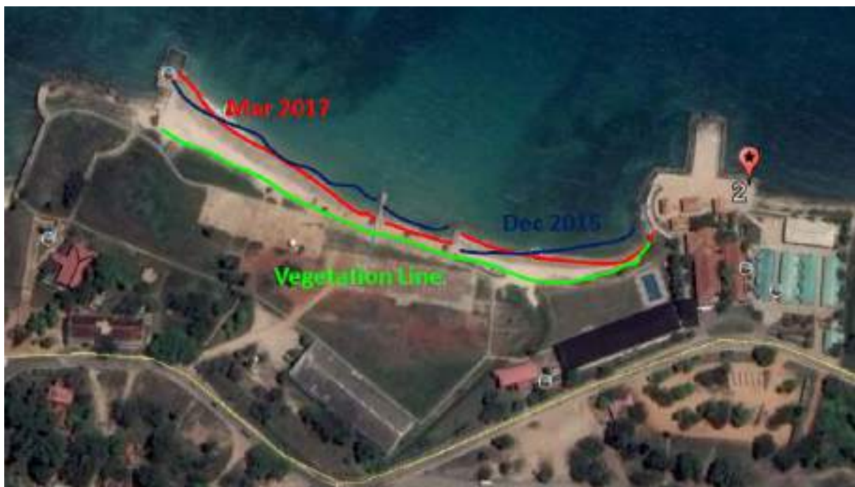
Figure 3.11: Shoreline variation in right hand side of the KKS port during the monsoons
