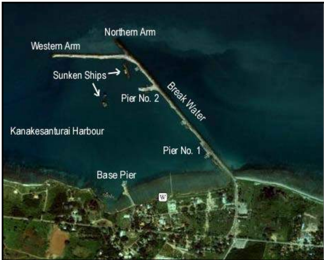
Figure 2.3: Layout of the Existing Kankesanturai Port, Jaffna
