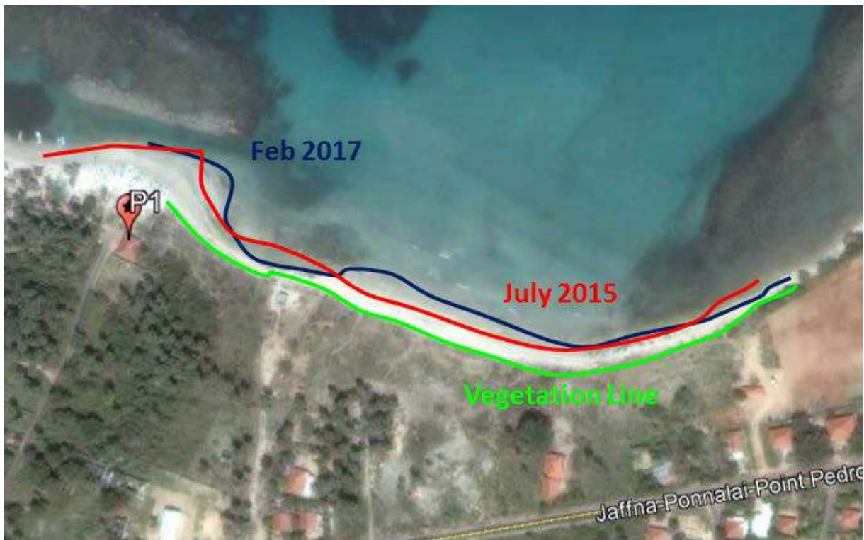
Figure 3.12: Shoreline variation in left hand side of the KKS port during the monsoons
